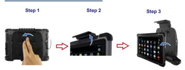
1.Slide the latch to open the hook
